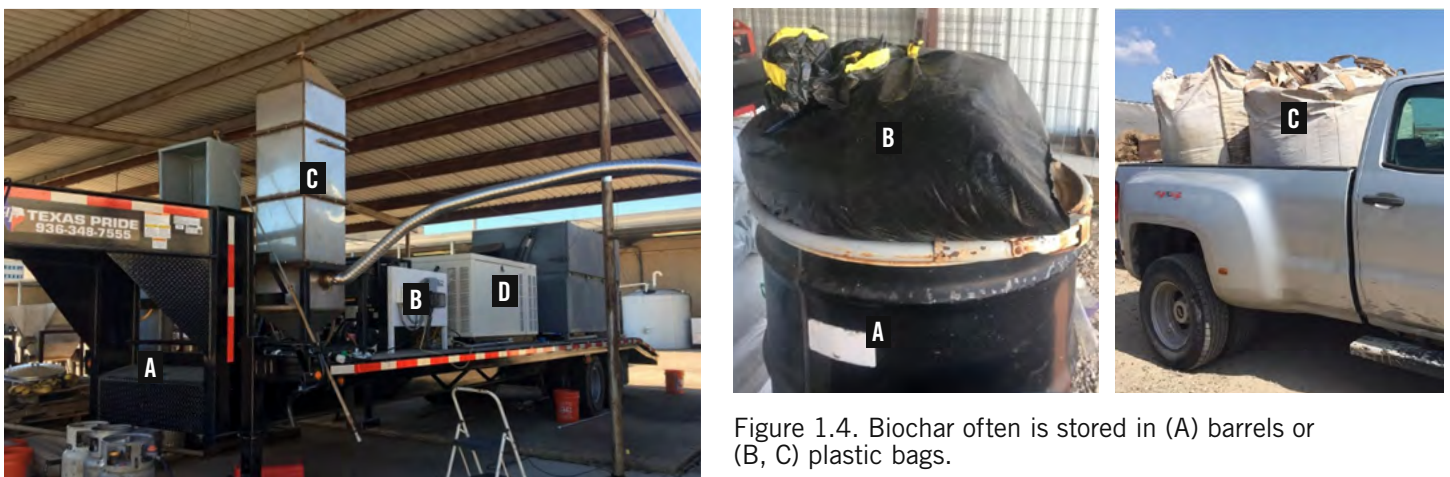
Figure 1.3. Biochar production system (Texas A&M University, College Station, TX) consisting of four main parts: (A) heating, (B) conditioning control, (C) biomass receptor and biochar collector, and (D) cooling system.
