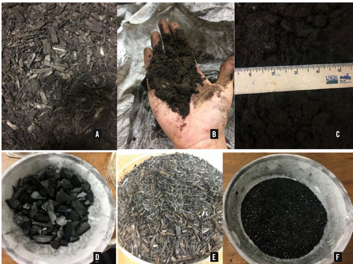
Figure 1.1. Biochar made from (A) fast pyrolysis at a temperature of 1022 °F from mixed hardwood; (B) sugarcane bagasse at 572 °F and (C) 842 °F; (D, F) pine wood chips (temperature not known); and (E) slow pyrolysis of sugarcane bagasse at a temperature of 662 °F.
