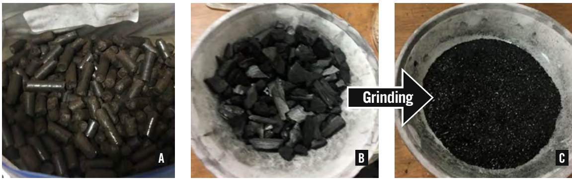
Figure 1.5. Biochar subjected to posttreatments: (A) pelletized biochar; (B) biochar from pine wood chips before posttreatment; and (C) after posttreatment (grinding).
